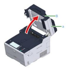
Press the button (A) and open the output tray (b) completely.
