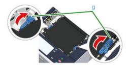
14 Hold the fuser unit handle and place the fuser unit into the machine.
