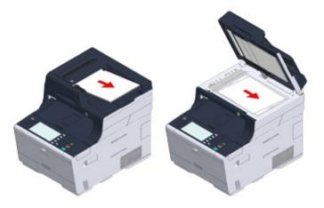
1 Hold the handle (B) and open the scanner unit (a) completely.
