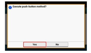
The machine starts searching for wireless LAN access points. The following screen is displayed for approximately 2 minutes, during which press and hold the WPS button for the wireless LAN access point for a few seconds.
