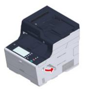
Siect the connector from the cover and connect with the wireless LAN module.
