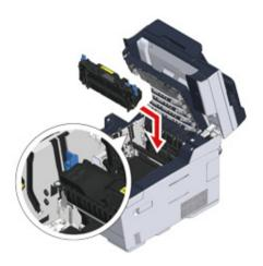
5 Tilt the lock levers (f) on the both sides of the fuser unit.
