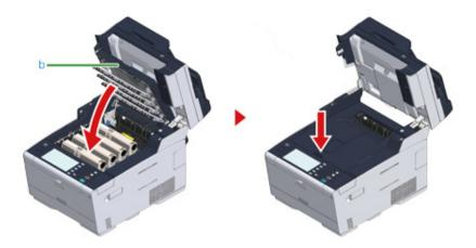
Hold the handle (B) to close the scanner unit (a).
