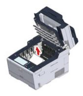
19 Hold the lock levers of belt unit and place the belt unit into the machine.
