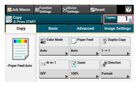
4 Enter the number of copies by using the numeric keypad or the numeric buttons.
