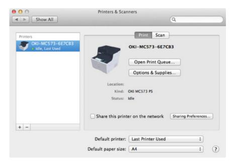
If [OKI MC573 PS] is not displayed for [Kind] correctly, click [-], delete the machine from [Printers], and then newly perform steps 8 to 12.
