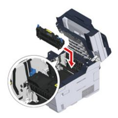
15 Tilt the lock levers (d) on the both sides of the fuser unit.
