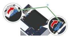
Hold the fuser unit handle and place the fuser unit into the machine.
