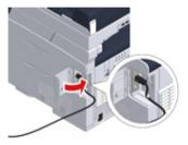
Insert the other end of the USB cable into the USB interface connector on the computer.
