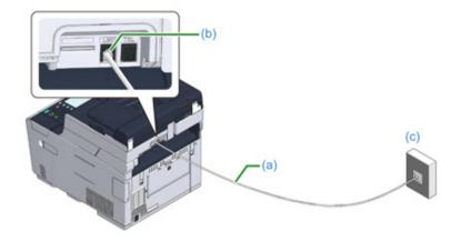
1 Plug one end of the included telephone cable (a) into the LINE connector (b) of the machine and the other end into a public line (analog) (c).
