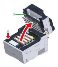
Remove the four image drums from the machine and place the image drums on a flat surface.
