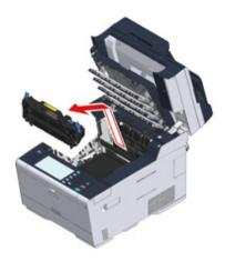
Turn the lock levers (e) on the both sides of the belt unit toward you and remove the belt unit by holding the lock levers.
