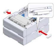
3 Slowly stack the machine on the additional tray unit aligning their back sides and right sides.
