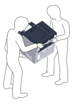
Do not open the scanner unit until step 4.
