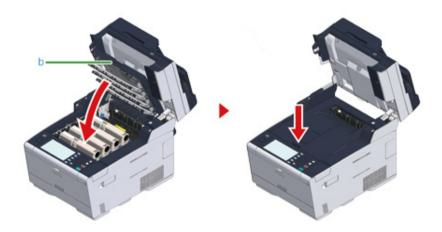
Hold the handle (B) and close the scanner unit (a).
