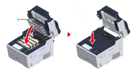
If the error message that the output tray is open does not disappear, make sure that the output tray is closed securely.
