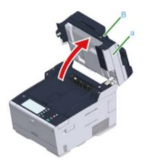
3 Press the button (A) and open the output tray (b) completely.
