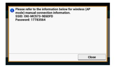
Enter the [SSID] and [Password] that you checked in step 10 to connect the machine and your wireless device.
