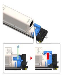
If you close the output tray without turning the blue lever when installing the toner cartridge into the image drum, it may cause a malfunction. Be sure to turn the blue lever until its top aligns on the lug in the back of the toner cartridge.
