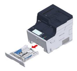
2 Slide the paper guide (a) to the width of paper to be loaded.
