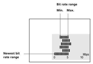
Indicates the transition of bit rate of the playback picture for a period up to the present.
