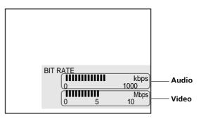
Bit rate refers to the amount of video/audio data per second in a disc. The higher the bit rate is, the larger the amount of data. When the bit rate level is high, there is a large amount of data. However, this does not always mean that you can get higher quality pictures or sounds.
