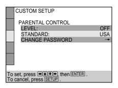
5 Select an area as the standard for playback limitation level using **↑**/**↓**, then press **→**.
