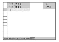
3 Input the time code using the number buttons, then press ENTER.
