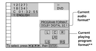
\* "PCM," "DTS,""DOLBY DIGITAL" or "MPEG" is displayed. In "DOLBY DIGITAL" case, the channels in the playing track are displayed by number as follows:
