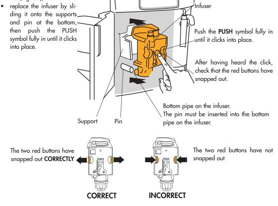
Check that the two red buttons have snapped out, otherwise the door cannot be closed.
