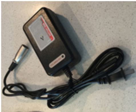
CHARGER Power charger with connection to joystick, and power cord to plug into the wall outlet
