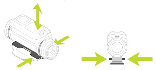
7. Adjust the position of the TomTom Bandit, then push the pitch mount lever to the closed position to lock the pitch mount.
