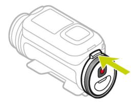
2. While holding the lever turn the cap anti-clockwise until you see two dots aligned.
