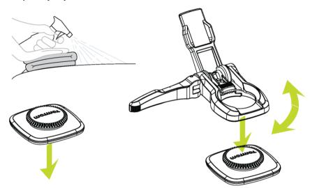
3. In dry, room-temperature conditions, attach the mount base. Push the mount base firmly down on to the surface.
