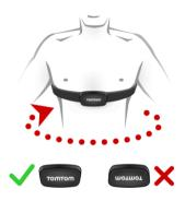
**Tip**: Wet the sensors on the inside of the strap before placing it around your chest. This makes it easier for the monitor to pick up your heartbeat.
