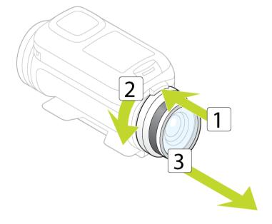
To install a lens cover, put the lens cover on the TomTom Bandit lens and turn it clockwise until it locks.
