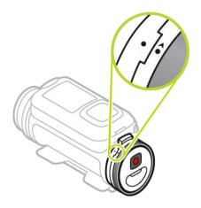
6. Turn the cap clockwise to lock the Batt-Stick into the camera.
