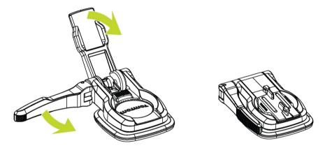
6. Install the TomTom Bandit on the 360 pitch mount. Make sure the TomTom Bandit is secure.
