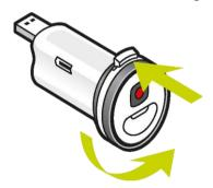
2. When you see a dot and arrow to the left of the release lever the Batt-Stick can be inserted as described above.
