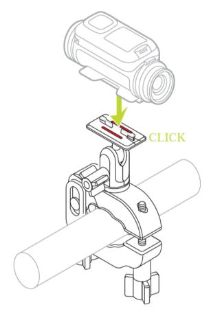
Install the bike mount only on a clean and dry surface. Wax, oil, dirt and moisture will reduce grip, causing the mount to move.
