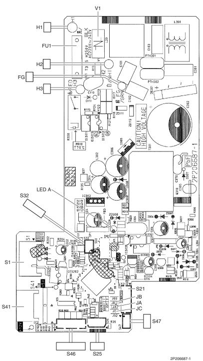
Printed Circuit Board Connector Wiring Diagram
