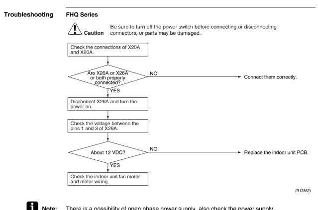
Note: There is a possibility of open phase power supply, also check the power supply.
