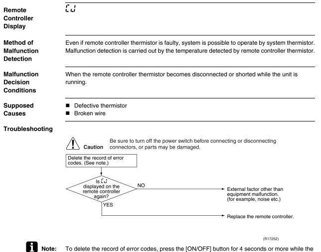
To delete the record of error codes, press the [ON/OFF] button for 4 seconds or more while the error code is displayed in the inspection mode.
