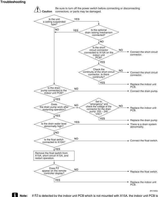
If ℜ∃ is detected by the indoor unit PCB which is not mounted with X15A, the indoor unit PCB is defective.
