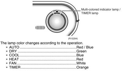
Brightness Setting The brightness of the multi-colored indicator lamp can be adjusted L (low), H (high), or OFF.
