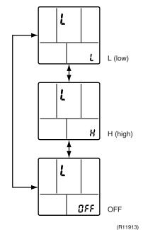
Press the [Mode] button for 5 seconds to exit from the brightness setting mode. (When the remote controller is left untouched for 60 seconds, it returns to the normal mode also.)
