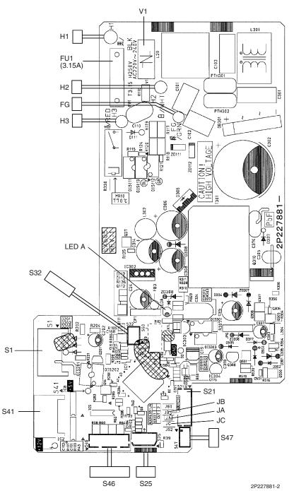
PCB (2): Signal Receiver PCB
