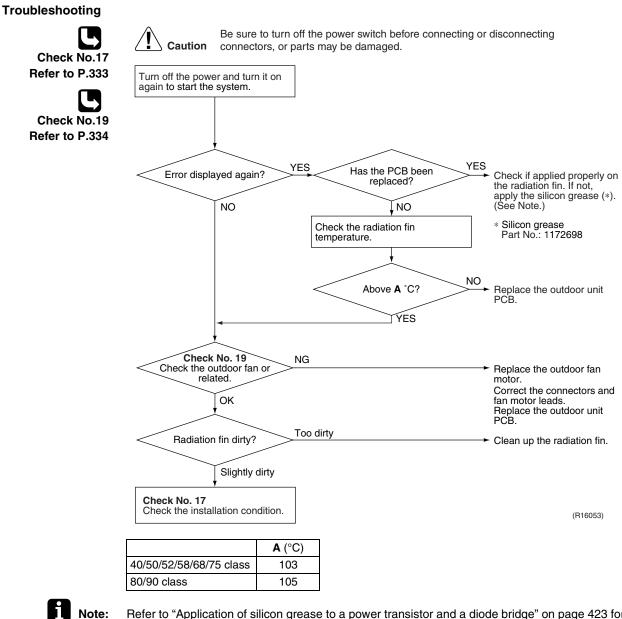
Refer to "Application of silicon grease to a power transistor and a diode bridge" on page 423 for detail.
