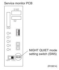
Install the removed jumper switch as described below. This jumper switch is needed later to disable this setting.
