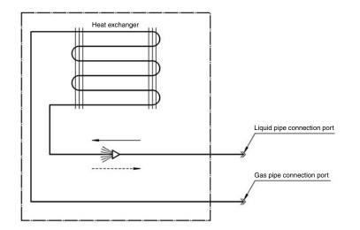
Refrigerant flow Cooling → Heating - →
