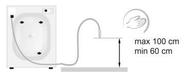
The drain hose is at the back of the machine. Fix the drain hose so that it does not move while the machine is in operation (use the elbow as shown below). Do not place the hose too deep into the outlet pipe!
