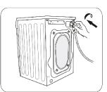
Use the new hoses supplied with the machine. Do not re-use old hoses.
