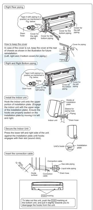
(This can be used for left rear piping and left bottom piping also.)
