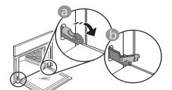
Simply remove the door by continuing to close it while pulling it upwards at the same time until it is released from its seating. Put the door to one side, resting it on a soft surface.
