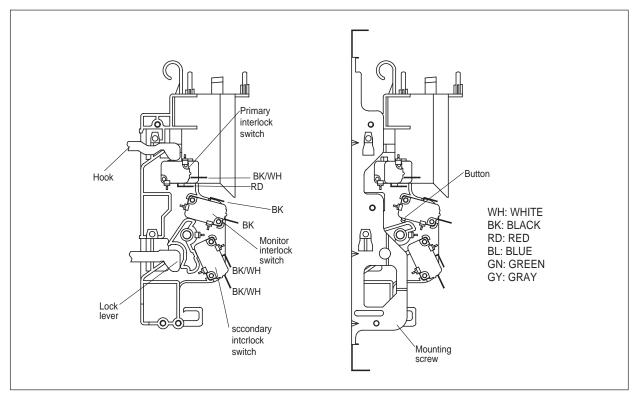
The door lock mechanism is a device which has been specially designed to completely eliminate microwave radiation when the door is opened during operation, and thus to perfectly prevent the danger resulting from the leakage of microwave.
