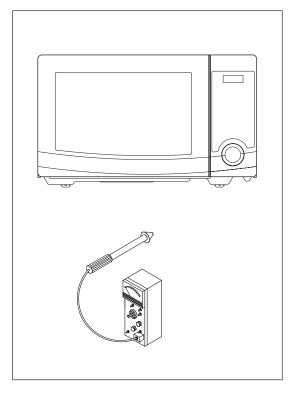
4) When measuring near a corner of the door, keep the probe perpendicular to the areas making sure the probe end at the base of the cone does not get closer than 2 in. from any metal. If it does not, erroneous reading may result.
