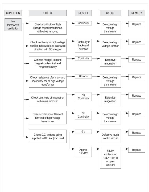
(TROUBLE 3) No microwave oscillation even though fan motor rotates.
