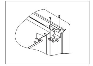
**NOTE** : After replacing the door assembly, perform a check of correct alignment with the hinge and cavity front plate.
