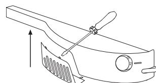
In case the fridge is equipped with an overhead light as shown below (figure A or figure B), take the above steps in order to replace the light bulb: using a screwdriver, remove the protective transparent cover, widening the wings. Replace the light bulb, reposition the protective cover and power up the appliance.
