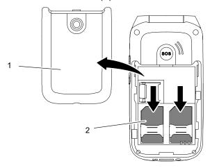
The battery compartment contains a useful diagram which indicates how to position and align the SIM card correctly in the compartment.
