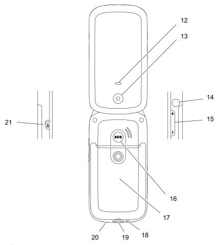
12 LED (for missed events) 13 Camera 14 Headphone connection port 15 Volume key, increase / decrease SOS (emergency call) key 16 17 Battery compartment cover 18 Charge contacts USB connection port 19 20 Torch (LED) Torch switch 21
