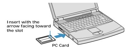
Do not force a PC Card into the slot as this may damage the connector pins.
