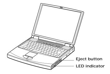
Do not push the eject button when the LED indicator is turned on. Otherwise, data may be lost.
