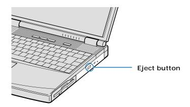
**3** Place an optical disc on the tray with the label side facing up. For DVDs that can be played on both sides, the side of the disc facing up is the side that plays.
