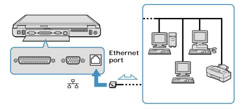
Warning: Only connect 10Base-T and 100Base-TX cables to the  $\frac{P}{D}$  Ethernet port. Do not connect any other type of network cable or any telephone line. Connecting cables other than those listed above may result in an electric current overload and could cause a malfunction, excessive heat, or fire in the port. To connect the unit to the network, contact your network administrator.
