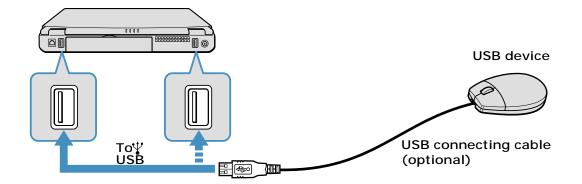
You can use an optional Sony USB mouse such as the PCGA-UMS1 series (not supplied) with this notebook. Since the USB mouse software driver is preinstalled in the notebook, you simply plug the USB mouse into the USB port to use it. One USB port supports one USB device.
