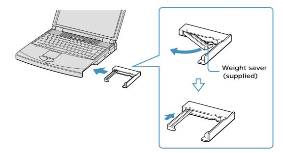
3 Manually lock the weight saver's release lever.
