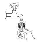
The appliance must be connected to the water mains using new hose-sets. The old hose-sets should not be reused.
