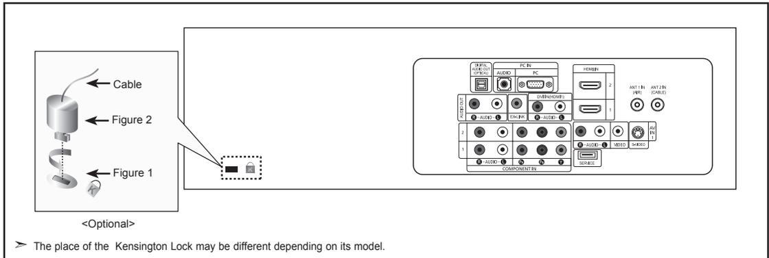
1. Insert the locking device into the Kensington slot on the LCD TV (Figure 1), and turn it in the locking direction (Figure 2).
