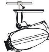
Mounted on truss
