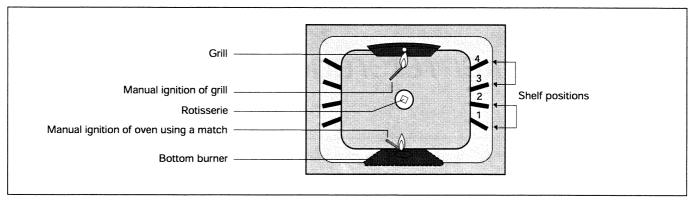
A single thermostat knob controls the operation of either the oven or the grill.
