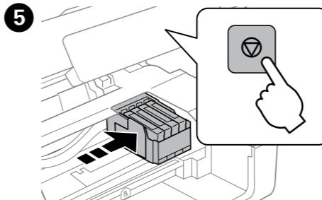
Press  $\diamond$  again to move the print head to the ink cartridge replacement position.
