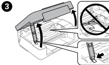
Open the scanner unit and press  $\diamond$ . The print head moves. If the print head does not move, hold down  $\diamond$  for 6 seconds or more until it moves.
