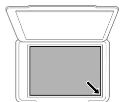
Open the document cover and place your original face-down on the scanner glass. Align the original with the front right corner of the glass.
