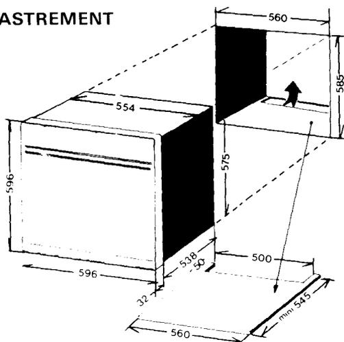
DANS LE CAS D'UN FOUR MONTÉ SOUS PLAN EN DUO AVEC UNE TABLE DE CUISSON, IL EST NÉCESSAIRE DE METTRE EN PLACE LE PANNEAU ISOLANT LIVRÉ EN OPTION.
