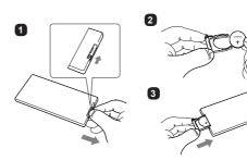
Replacing the battery (CR2025)
