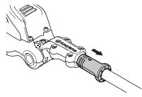
Tilt the cutting unit with its handle to the desired position.
