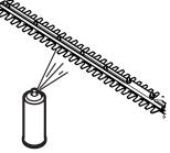
Ask your dealer for information on lubrication points and volume of grease in the gear. Use a high quality grease intended for Husqvarna products.
