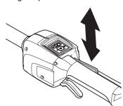
Check that the power trigger and the power trigger lockout move freely and that the return spring works properly.
