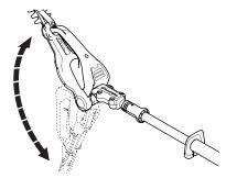
Release the position adjustment handle so that the cutting unit locks at the correct angle.
