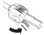
Press the power trigger lockout and make sure it returns to its original position when released.
