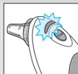
If you take the temperature of another person, the «ExacTemp» light (7) will be of help. It flashes during the measuring process as long as the probe is correctly positioned, and lights up continuously when an accurate reading has been taken.
