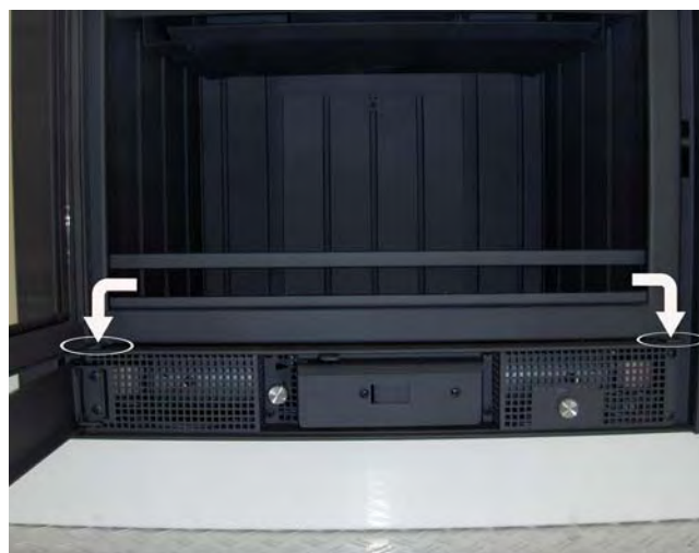
Illustration 7: Remove the 2 screws on the right and left bottom side.
