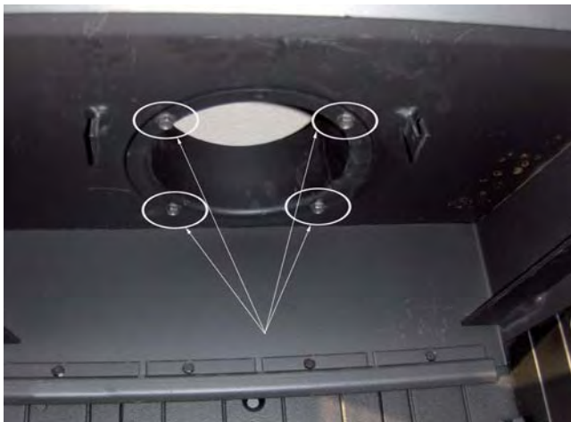
Illustration 1 Remove the pipe collar from the hearth
