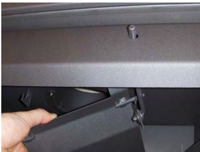
Illustration 1 Remove the pipe collar from the hearth
