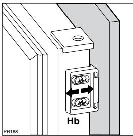
Fix cover (Hd) on guide (Hb) until it clips into place.
