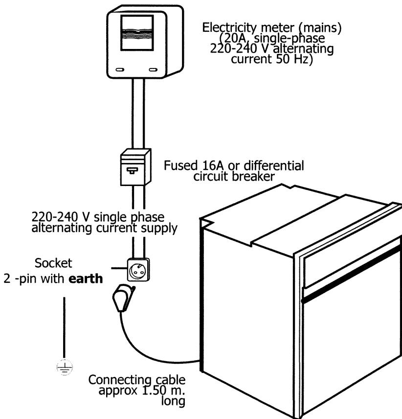
Before connecting your oven, make sure you are using the correct size cable. The cross-section should be the same as the cable connected to the oven. Use a 16-amp fuse.
