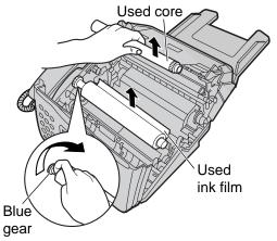
Remove the stoppers and tags from the new ink film. Find the "T" shaped gear (blue).
