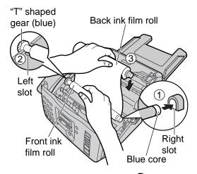
If the ink film is slack, tighten it by winding the gear.
