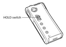
Slide the HOLD switch in the direction of the arrow.
