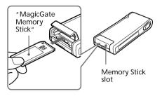
When the "Memory Stick" is inserted into the slot, "ACCESS" appears.
