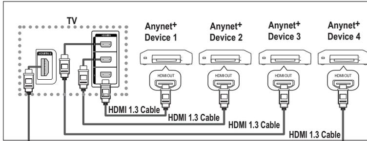
Connect the [HDMI IN 1], [HDMI IN 2], [HDMI IN 3] or [HDMI IN 4] jack on the TV and the HDMI OUT jack of the corresponding Anynet+ device using the HDMI cable.
