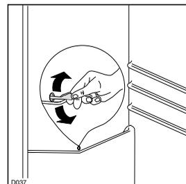
The freezer compartment, however, will become progressively covered with frost. This should be removed with a plastic scraper, whenever the thickness of the frost exceeds 4 mm. During this operation it is not necessary to switch off the power supply or to remove the foodstuffs.
