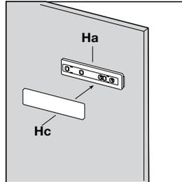
Open the appliance door and the furniture door at 90°. Insert the small square (Hb) into guide (Ha). Put together the appliance door and the furniture door and mark the holes as indicated in the figure. Remove the squares and drill holes with  $\varnothing 2$  mm at 8 mm from the outer edge of the door. Place the small square on the guide again and fix it with the screws supplied.
