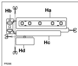
Place guide (Ha) on the inside part of the furniture door, as shown in the figure and mark the position of external holes. After having drilled holes, fix the guide with the screws supplied.
