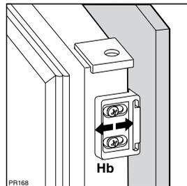
**After having reversed the opening direction of the doors check that all the screws are properly tightened and that the magnetic seal adheres to the cabinet. If the ambient temperature is cold (i.e. in Winter), the gasket may not fit perfectly to the cabinet. In that case, wait for the natural fitting of the gasket or accelerate this process by heating up the part involved with a normal hairdrier.**
