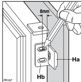
Should the lining up of the furniture door be necessary, use the clearance of slots.
