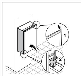
Fasten the appliance with 4 screws provided in the
