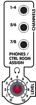
If you are sending the PHONES/CTRL ROOM signal to another piece of audio equipment, use a TRS cable (in this case to be used as a stereo cable), as the left and right channel signals are present in the PHONES/CTRL ROOM jack. If a mono cable is used, the left channel signal will get shorted to ground by the mono cable inside the jack. This could result in the headphone amplifier becoming hot and the right channel audio signal becoming distorted.
