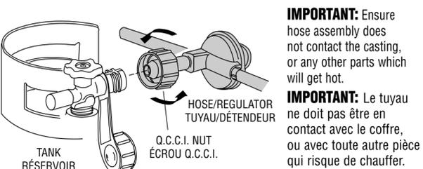
**IMPORTANT:** Ensure hose assembly does not contact the casting, or any other parts which will get hot.
