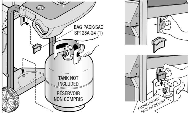
**IMPORTANT:** Ensure hose assembly does not contact the casting, or any other parts which will get hot.
