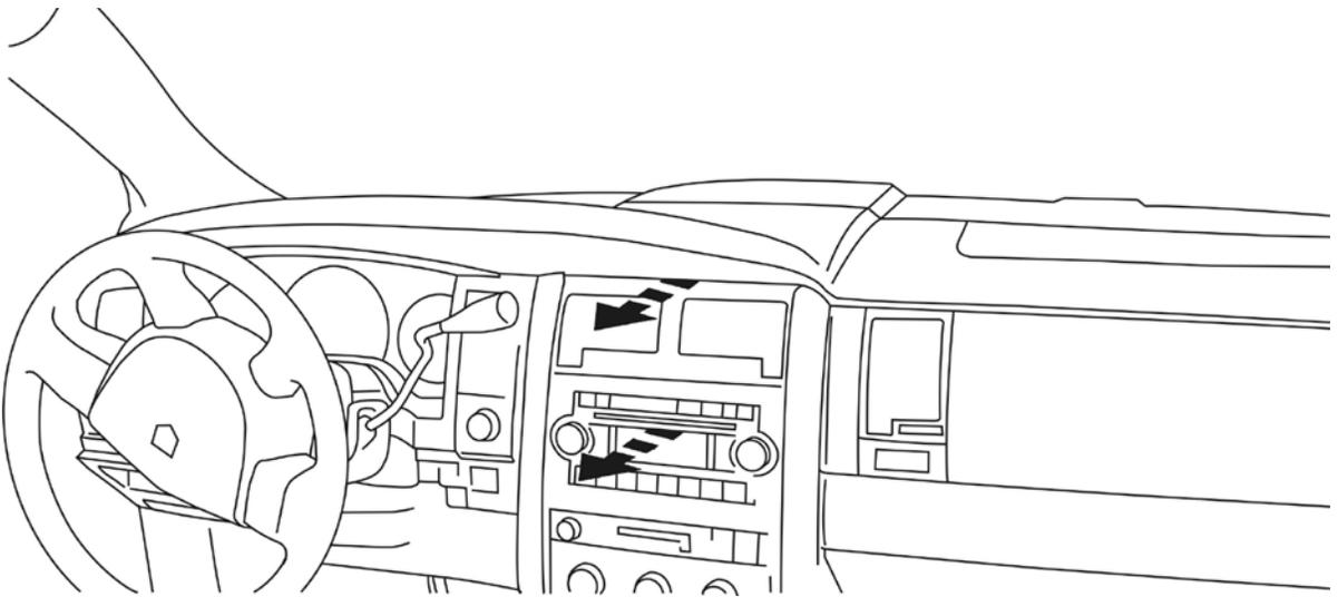
Remove trim panel and radio. ♦ Retirez le panneau de garniture et la radio.
