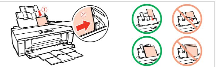
Load the paper with the printable side up.
