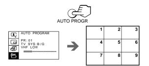
The TV starts scanning and presetting channels automatically. When all of the receivable channels are stored, the AUTO PROGRAM menu disappears and the first nine preset TV programs appear on the nine sub screens. The nine sub screens disappear after being displayed for several seconds.
