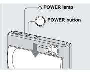
Slide the lens cover in the direction of arrow or press the POWER button.
