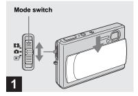
Set the mode switch to 1, and slide the lens cover to turn on the power.
