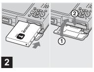
➡ Install the battery pack, then close the battery/"Memory Stick Duo" cover.
