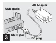
→ Connect the AC Adaptor (supplied) to the DC IN jack of the USB cradle (supplied).
