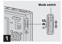
→ Set the mode switch to ▲, and slide the lens cover to turn on the power.
