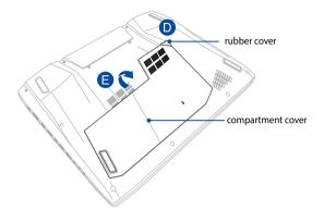
F. Remove the screws that secures the HDD bay to the compartment.
