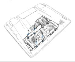
G. Disconnect the HDD bay from the HDD port then remove the HDD bay from the compartment.
