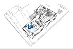
N. Secure the HDD and drivebay assembly with the screws that you removed in step F.
