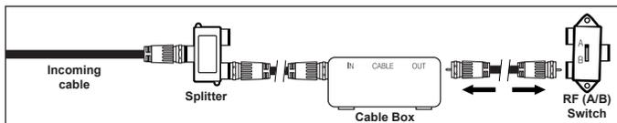
5. Connect another cable between the other OUT terminal on the splitter and the A-IN terminal on the RF (A/B) switch.
