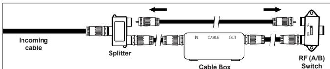
6. Connect the last RF cable between the OUT terminal on the RF (A/B) switch and the ANT IN terminal on the rear of the TV.
