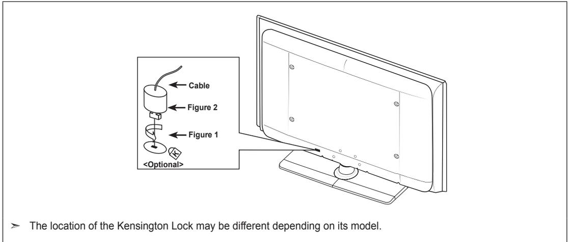
1. Insert the locking device into the Kensington slot on the LCD TV (Figure 1) and turn it in the locking direction (Figure 2).
