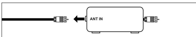
2. Connect this cable to a two-way splitter.
