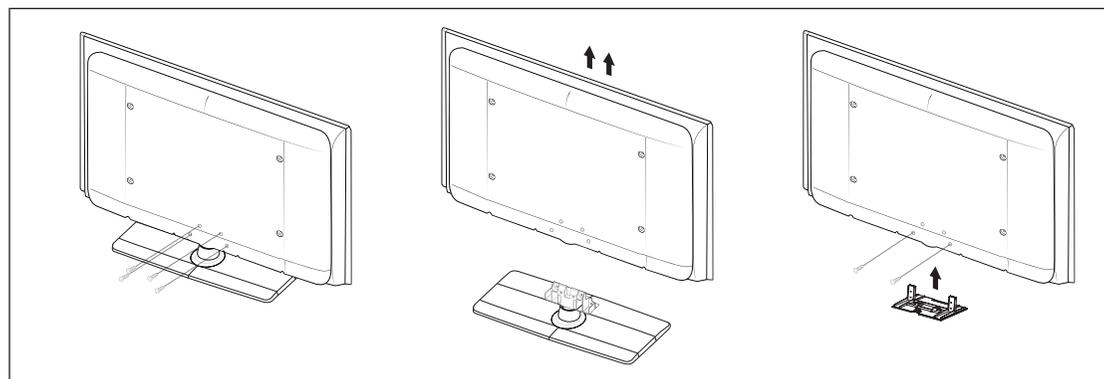
1. Remove four screws from the back of the TV.
