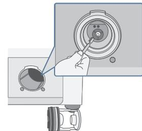
8. Close up the opening of drain tube with cap.
