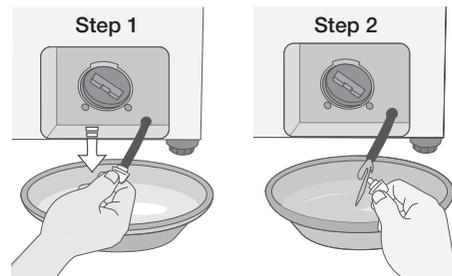
4. Remove the debris filter cap.
