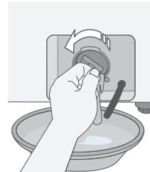
5. Wash any dirt or other material from the debris filter. Make sure the drain pump propeller behind the debris filter is not blocked.
