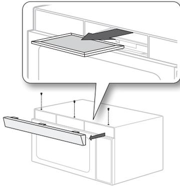
6. Slide a new charcoal filter into place. The filter should rest at the angle shown.
