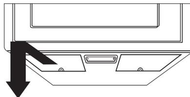
2. Soak the grease filter in hot water and a mild detergent. Rinse well and shake to dry. Brushing the filter lightly can remove embedded dirt.
