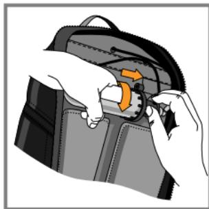
**Check that the cartridge is screwed in tightly before each use of the airbag to avoid leakage and malfunctions.**
