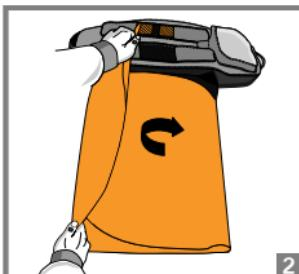
3. Now fold the bottom part of the airbag. The airbag width must correspond to the width of the airbag compartment.
