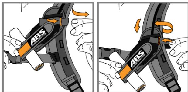
In order to adjust the height open and undo the Velcro closure, attach the handle plate to the appropriate plastic grommet and fasten the Velcro closure.
