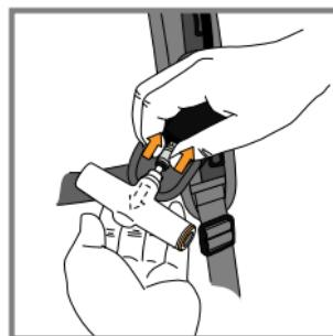
Remove the handle when ABS backpack is not in use and store it in the pocket located at the hip strap.
