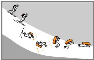
The moving snow flushes large volume objects to the surface. If these objects have a smaller dimensional weight than the surrounding snow, they will stay at the surface.
