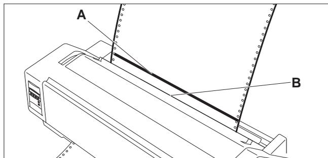
The bottom edge of the currently valid first printing line **A** of the paper is transported to the tear edge **B**.
