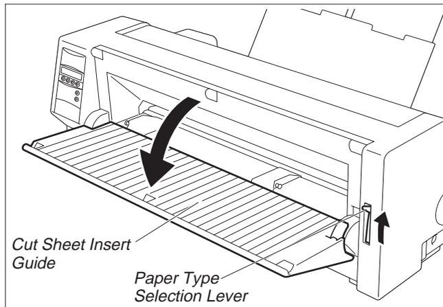
Set the Paper Type Selection Lever to Cut Sheet Paper mode. Make sure that the printer is in Single Sheet mode. For how to select Single Sheet mode refer to page 14 (*Paper path quick selection*).
