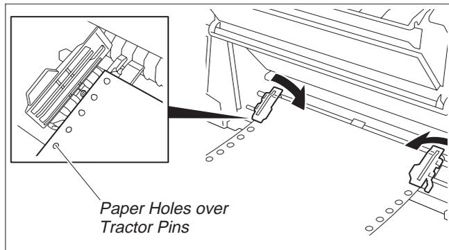
With the printing side of the paper facing up, fit the feeding holes on the left edge of the paper over the Left Tractor pins and close the Paper Flap.
