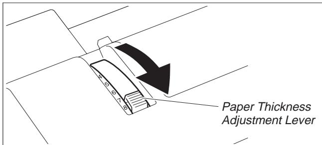
Set the Paper Thickness Adjustment Lever to the “8” position.
