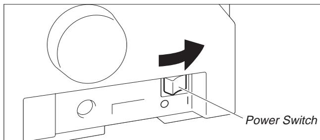
Turn the Power Switch of the printer ON ("I").
