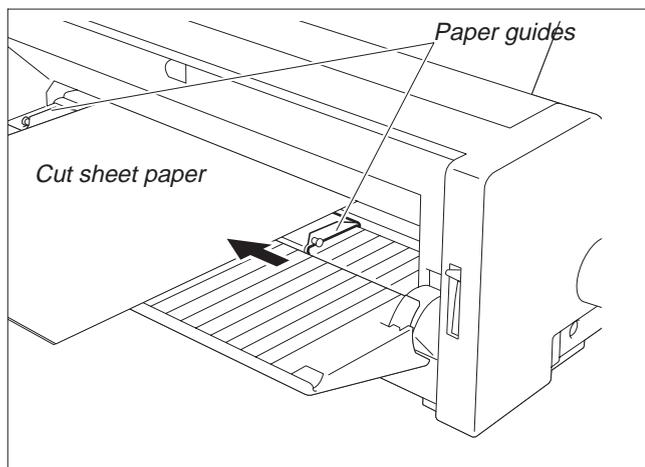
Place a sheet of paper aligned to the Left Paper Guide, and adjust the Right Paper Guide to the right edge of the paper. Insert the paper between the Left and Right Paper Guides. The paper is automatically fed to the print start position and the printer is ready to print.
