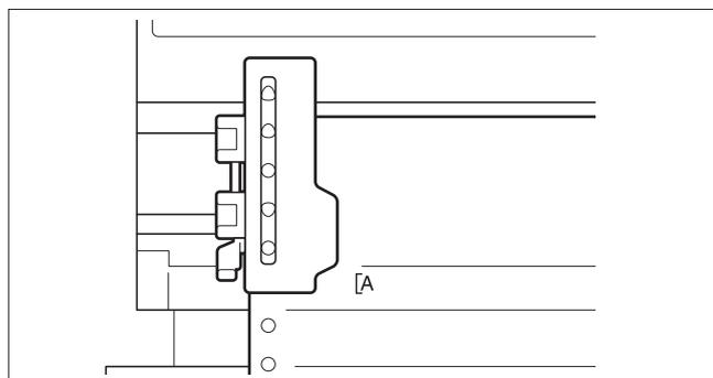
After the paper is set, adjust the left margin by moving the Tractors left or right. The “[A]” mark is the standard print start position.
