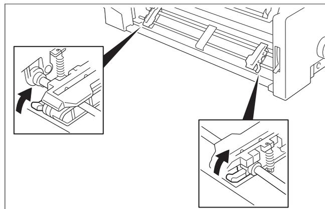
Stand the Left and Right Tractor Fixing Levers up (in the direction indicated by the arrow), and release the locks.
