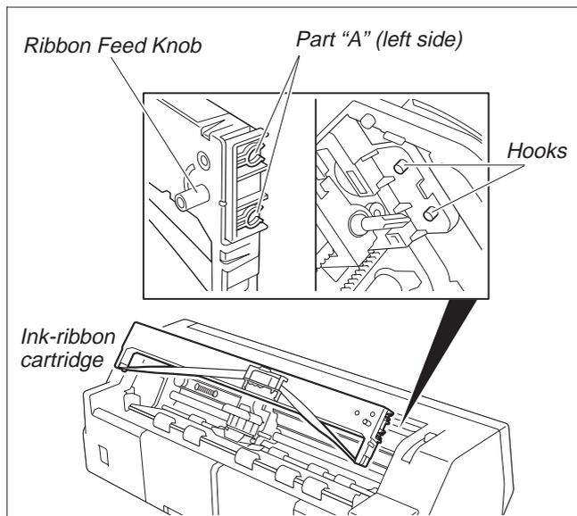
Align the part "A" on the left side of the Ink-ribbon Cartridge to the two hooks of the printer, push the cartridge all the way until it clicks. If there is resistance, push it while turning the Ribbon Feed Knob.
