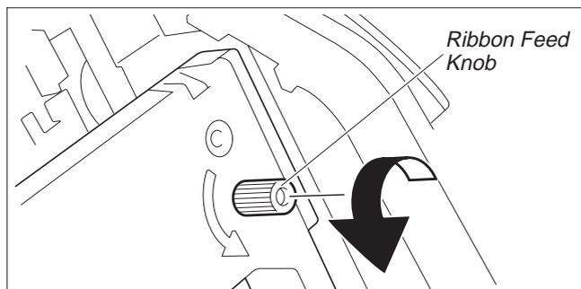
Turn the Ribbon Feed Knob in the direction indicated by the arrow to remove any slack in the ribbon.
