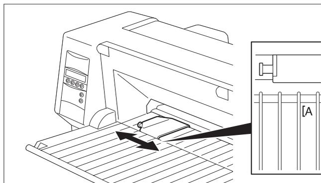
Determine the left margin by moving the Left Paper Guide left or right. (The “[A]” mark indicates the standard print start position.)
