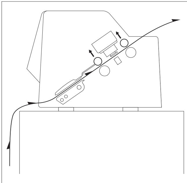
If frequent forward and return feed movements will be performed with fanfold paper, you should position the printer as illustrated in the figure.
