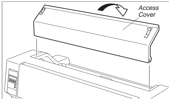
When the Ink-ribbon Cartridge setting is complete, attach the Access Cover.
