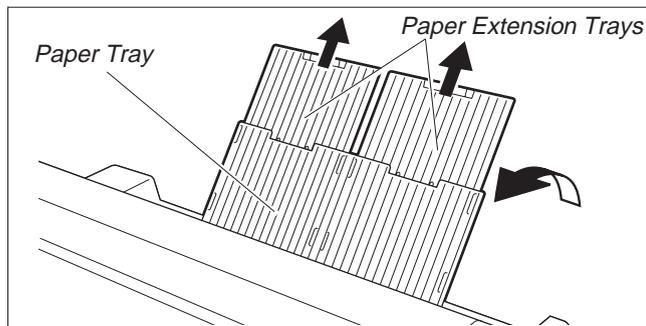
Stand the Paper Tray up in the direction indicated by the arrow. While holding the Paper Tray, pull up the Paper Extension Trays.
