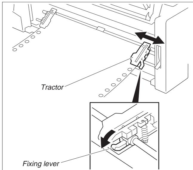
Push down the Left Tractor Fixing Lever to lock the Left Tractor.
