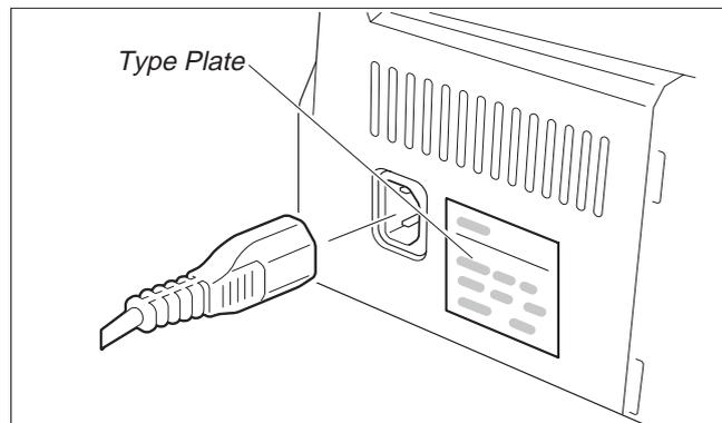
Make sure that the unit is set to the correct voltage (i.e. 230 V for Europe, 120 V for the USA). Refer to the type plate beside the power inlet on the rear side of the printer.
