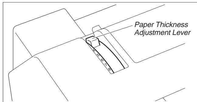
To obtain optimum print quality, the gap between the Print Head and the Platen needs to be adjusted according to the thickness of the paper to be used.
