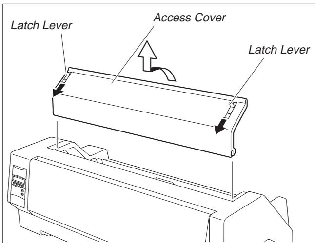
Pull the Latch Levers near the right and left ends on the Access Cover to the front, and detach the entire Access Cover.
