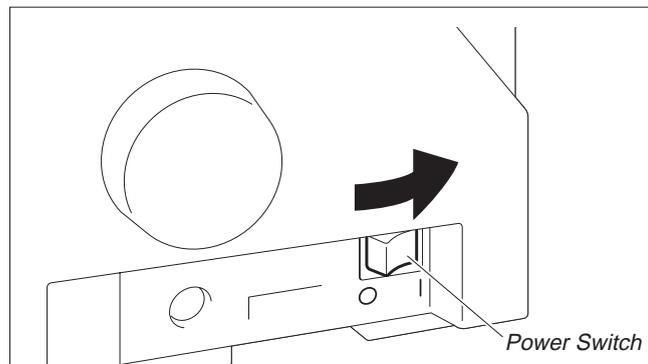
The power switch, which is used for switching the printer on and off, is located at the right side of the printer.
