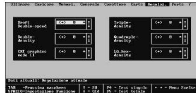
The above window is used to test and adjust the vertical alignment of the printer in each printing mode. You may never have to use the procedure described in this section, but after you have been using your printer for some time you may find that the dots of some graphics do not align correctly. For example, what should look like:
