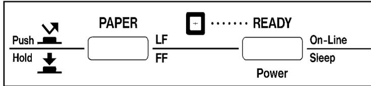
The control panel gives you push-button control over the printer's power and paper feed operations. It also includes an indicator light that tells you the current status of the printer at a glance.
