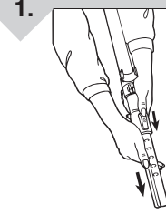
Diagram 1 Connect metal wand to the hose and extend to desired length.
