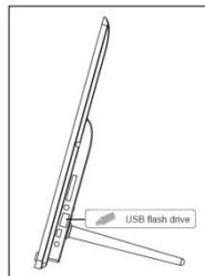
USB data carriers can only be plugged into the USB slot in one direction.
