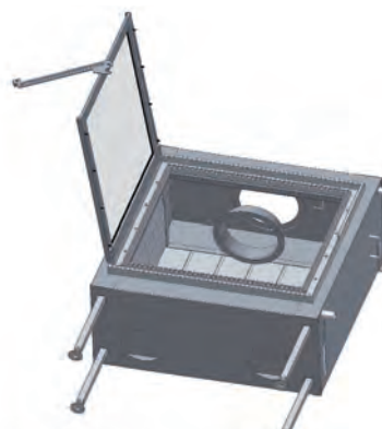
Illustration 1 Removing the flue collar from the stove
