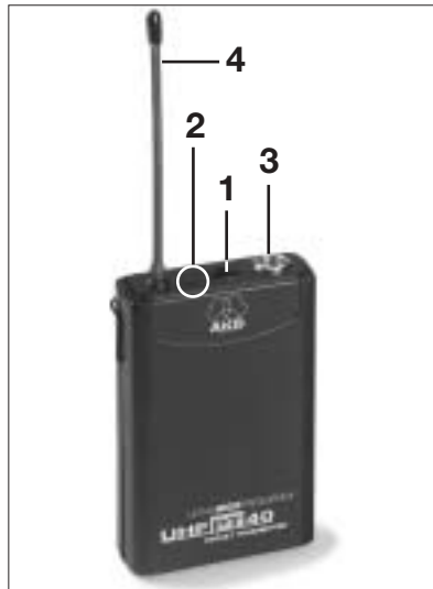
Fig. 1: Top panel controls
