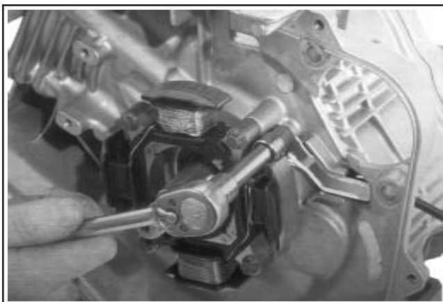
Figure 11-56. Installation du blindage.
