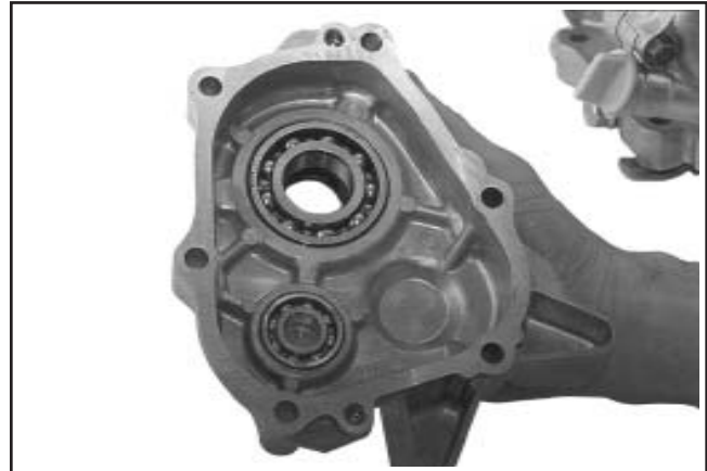
Figure 11-25. CS8.5-12. Installation du palier.
