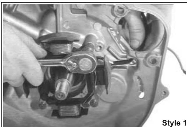
Figure 11-56. Installation du blindage.
