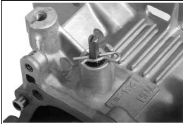
Figure 11-6. CS4, CS6. Installation du clip.
