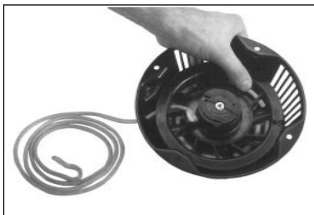
Figure 7-5. Installation de la corde.
