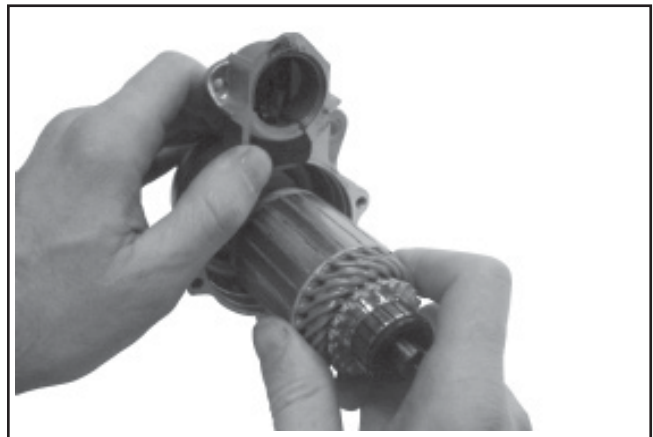
Figure 8-63. Installation de l'armature.
