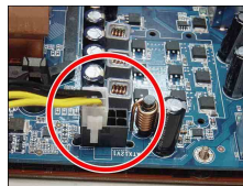
Plugged from a 4-pin ATX12V power.
