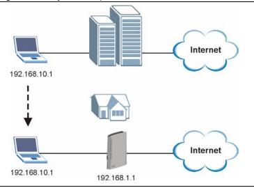
The Any IP feature does not apply to a computer using either a dynamic IP address or a static IP address that is in the same subnet as the ZyXEL Device's IP address.
