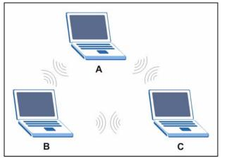
Figure 213 Peer-to-Peer Communication in an Ad-hoc Network
