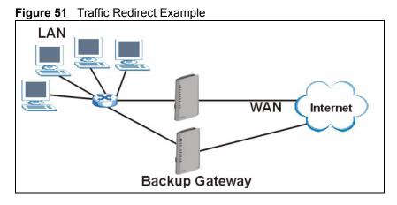
The following network topology allows you to avoid triangle route security issues when the backup gateway is connected to the LAN. Use IP alias to configure the LAN into two or three logical networks with the ZyXEL Device itself as the gateway for each LAN network. Put the protected LAN in one subnet (Subnet 1 in the following figure) and the backup gateway in another subnet (Subnet 2). Configure filters that allow packets from the protected LAN (Subnet 1) to the backup gateway (Subnet 2).
