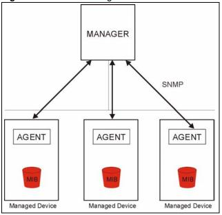
An SNMP managed network consists of two main types of component: agents and a manager.
